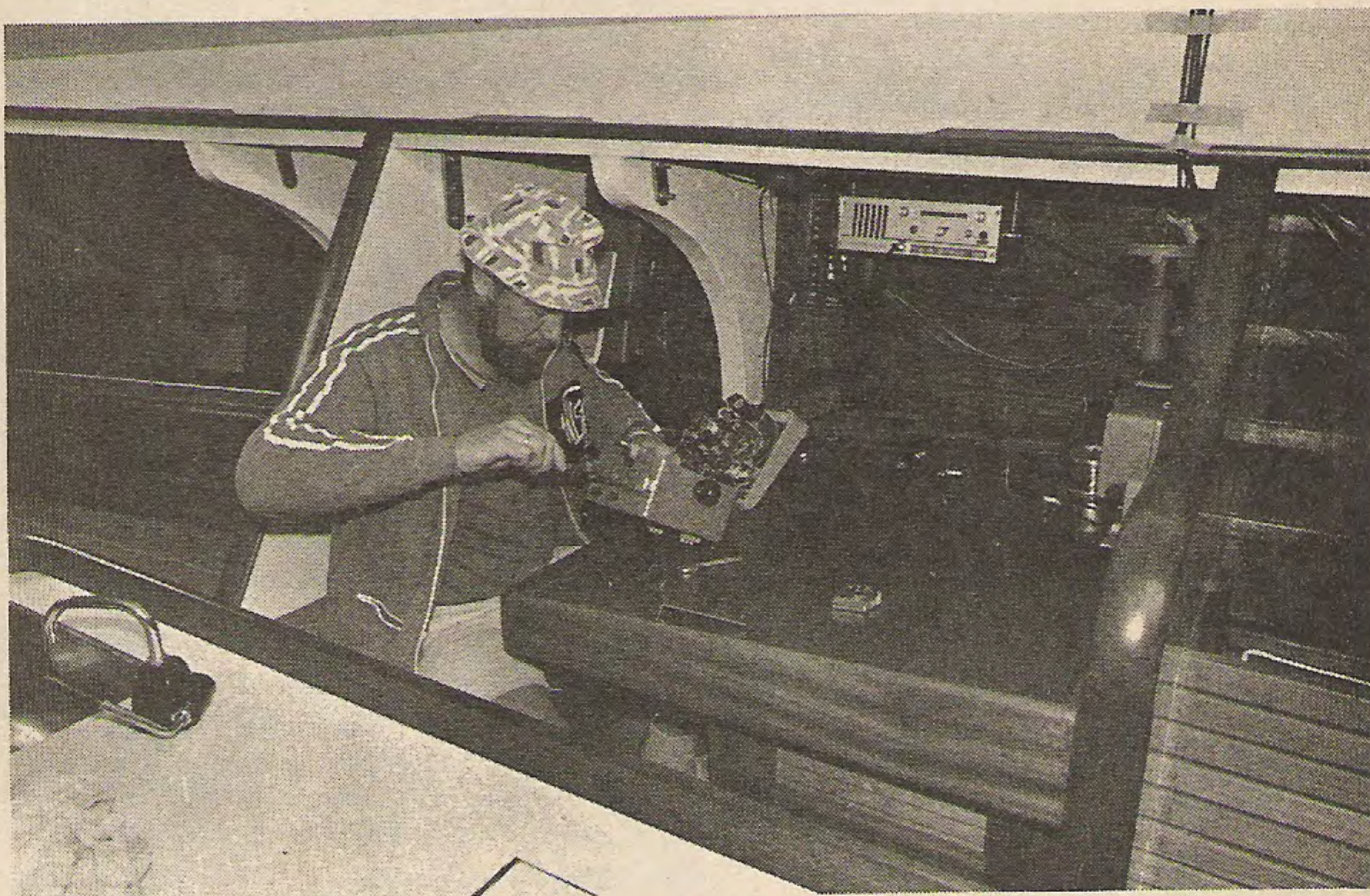
Navigator Jazz Jaspers at the navigation table. Behind him can be seen the chainplates placed well inboard and fastened below decks to steel brackets which carry the load down the topsides
